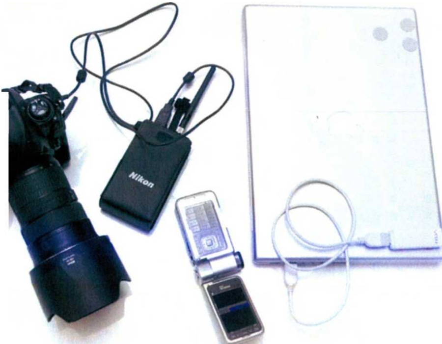
Camera, transmitter, computer, 3G-modem and mobile are essential for sending pictures.
